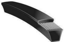
Industrial V-belts include the common, narrow, wide, largeangle and speed-change V-belt. The common and narrow V-belts are the most frequently used. With a new material-polyester wire rope being its tension element, the polyester wire-rope V belt features high strength, low elongation rate, long life utility, stable dimension, high bending and wearing resistance, etc., thus better satisfying the requirements for mechanical transmission.
